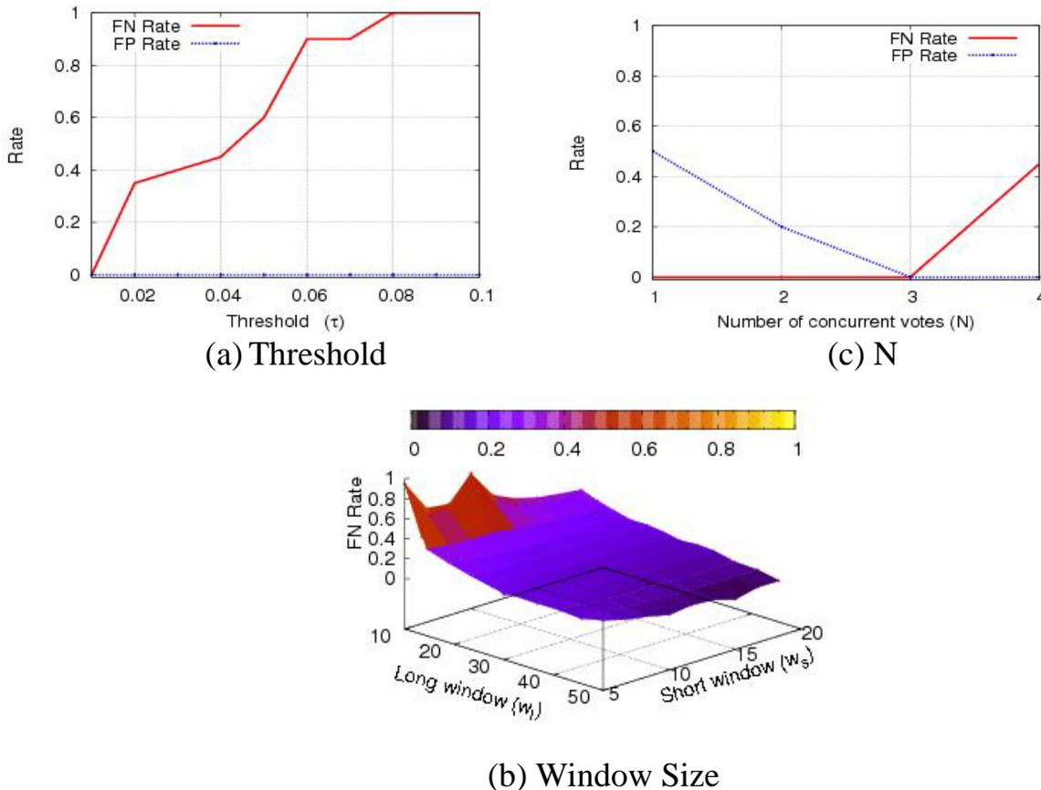
**Figure (4):** Effect of different parameters on the moving average detection technique.
