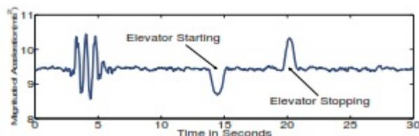
Figure 1: Accelerometer signature inside an elevator (caused by the elevator starting and stopping).
