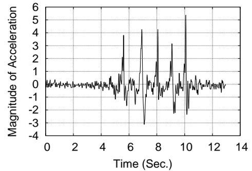
Fig. 3: The acceleration pattern for five steps.
