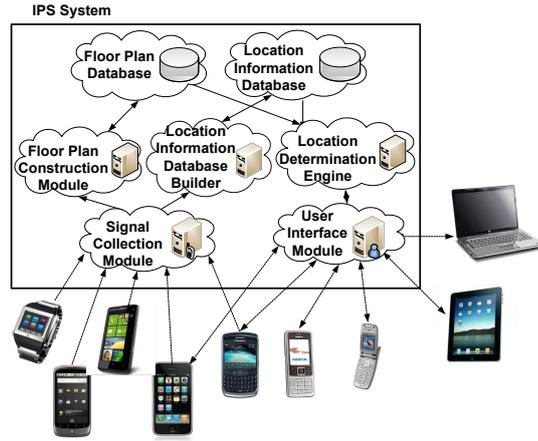
Fig. 1: The IPS system architecture.
