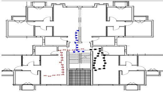
Fig. 2: An example of the different traces generated by the different users using the cell phones' inertial sensors.
