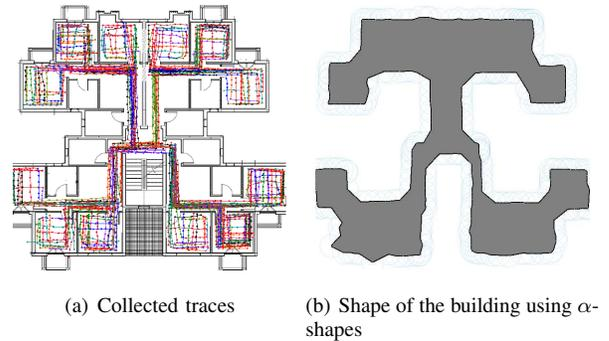
Figure 2. Construction of the overall building floor-plan from multiple motion traces (a). The grey area in subfigure (b) represents the estimated floor-plan shape.
