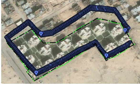
Figure 8. Trace of user's motion estimated by dead reckoning
