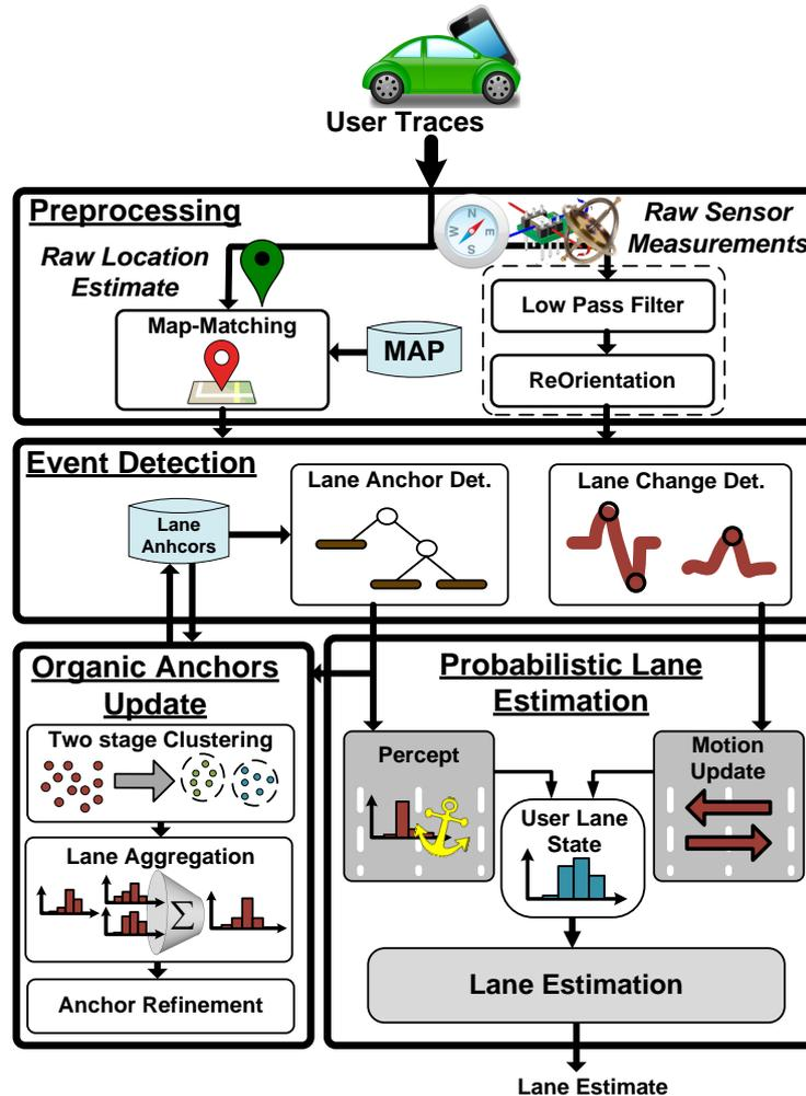
Figure 2. *LaneQuest* system architecture. *LaneQuest* predicts the car current lane using a probabilistic approach by fusing knowledge of the car lane changes and a repository of lane-level anchors. Crowd-sourced traces are also used to detect new anchors and identify their lane position in an organic way.
