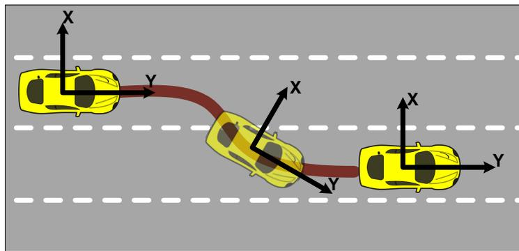
Figure 7. A car doing a lane change will have to make a small rotation around the z-axis, leading to a change in its x-axis acceleration.
