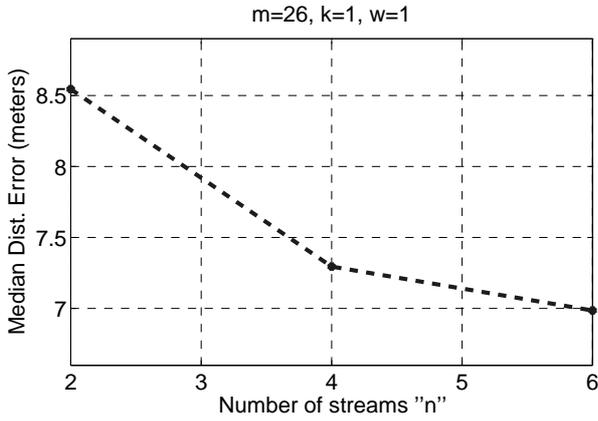
**Figure 8: Median distance error of the discrete space estimates versus the number of used raw data streams  $n$ . For a given  $n$ , the figure reports the best median distance error over all the  $\binom{6}{n}$  raw streams combinations.**
