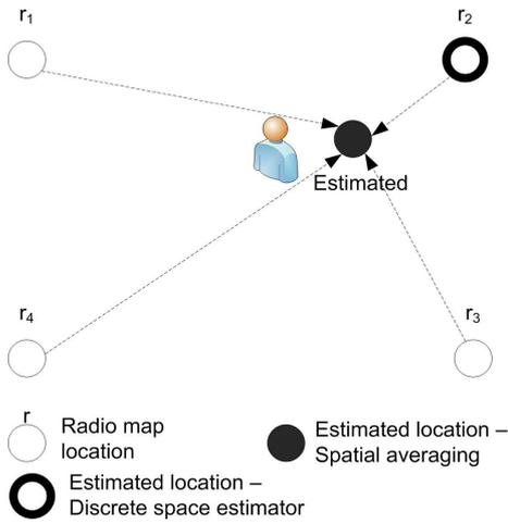
**Figure 4: An example of using the spatial averaging technique to enhance accuracy. The discrete space estimator will return the location  $r_2$  as it is the nearest to the actual user location. Using the spatial averaging technique, a better location estimate can be obtained by calculating the center of mass of the top 4 locations ( $k = 4$ ).**
