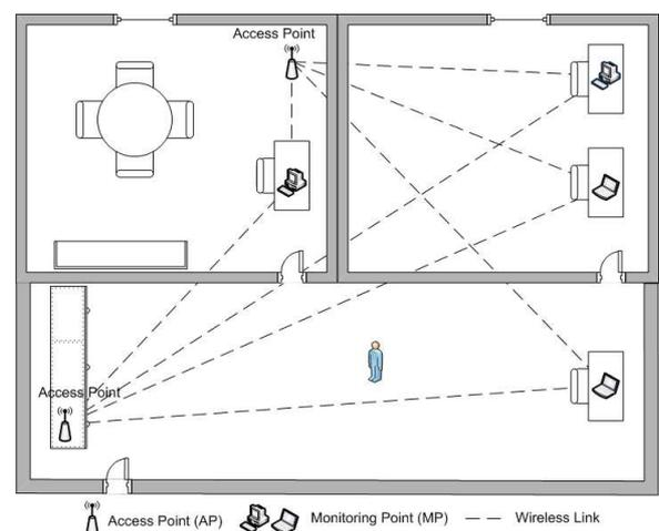
**Figure 1: An example of the different components of a device-free passive localization system. APs represent signal transmitters. Standard laptops and wireless-enabled desktops represent MPs. Any device can be used as an application server.**
