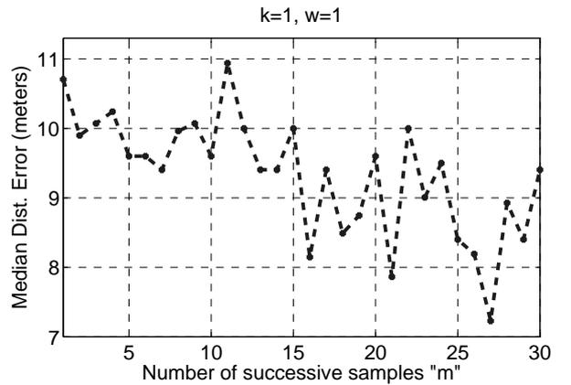
**Figure 7: Median distance error of the discrete space estimator for different values of the number of successive samples from each stream per location estimate ( $m$ ).**
