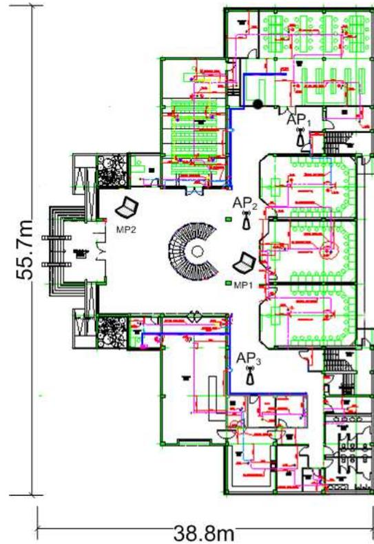
**Figure 5: Floor plan of the area where the *DfP* experiment was performed. The environment is rich in multipath, where furniture, plants, and substantial amount of metal exist. The figure also shows the locations of APs and MPs.**
