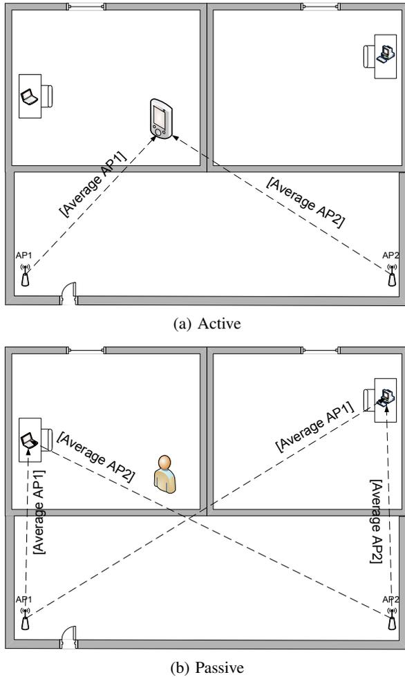
**Figure 3: Difference between active and passive radio maps' construction. In a passive radio map, we have a mean value per raw data stream, as compared to a mean value per AP. Also, a user does not carry any device when constructing the passive radio map.**
